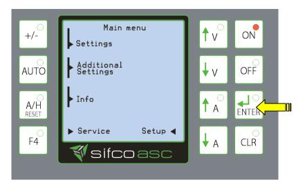
Select the desired menu point by pressing the corresponding key.
