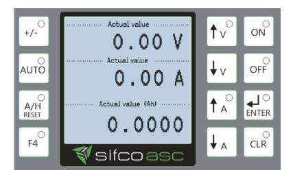
In normal operating mode, the digital display shows the actual current and voltage parameters of the DC power supply.
