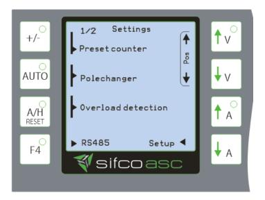
Select the desired sub item of the menu point by pressing the corresponding key.
