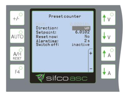
Select the desired item of the menu point "preset counter" by using the arrow keys.
