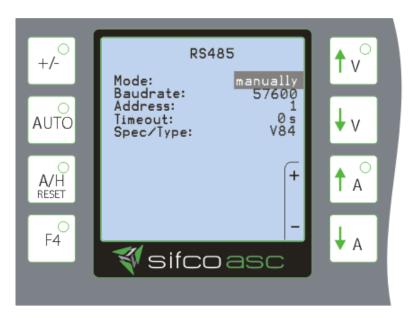
Select "manually" or "auto" mode by using the Up / Down keys.
