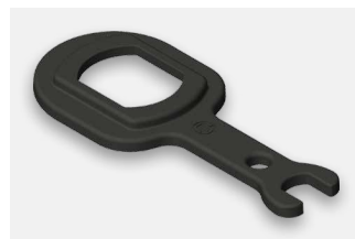
Mounting Wrench SL for opening and closing the terminal cap of small terminal casings LC and the lead screw fixing. Material: Grivory GVN
