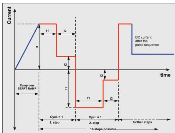
Examples: pulse shapes, schematic display
